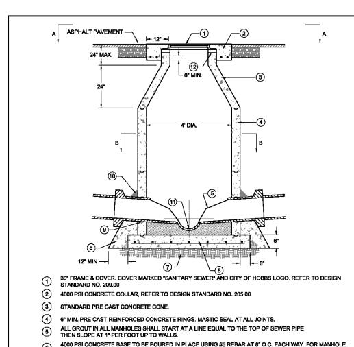
4000 PSI CONCRETE BASE TO BE POURED IN PLACE USING #5 REBAR AT 8" O.C. EACH WAY. FOR MANHOLE DEPTH, FROM RIM TO INVERT, OF UP TO 16' AND MAXIMUM PIPE DIAMETER OF 24". COMPACT BACKFILL UNDER ALL MANHOLES TO 95% MODIFIED PROCTOR DENSITY.
