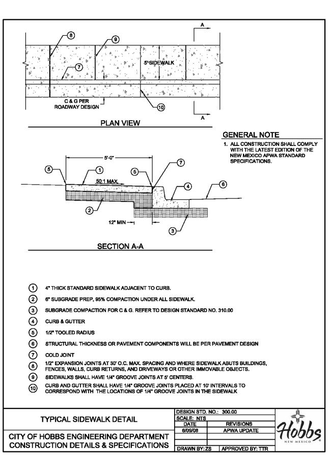
SIDEWALK TO BE INSTALLED ADJACENT ALL NEW CURB & GUTTER.
